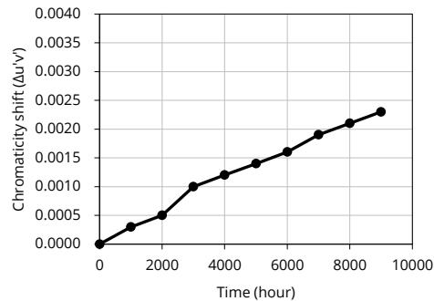
$T_s = 85^\circ\text{C}$ ,  $I_F = 300\text{mA}$ , RH < 65%, reported L70 > 54000 hours
