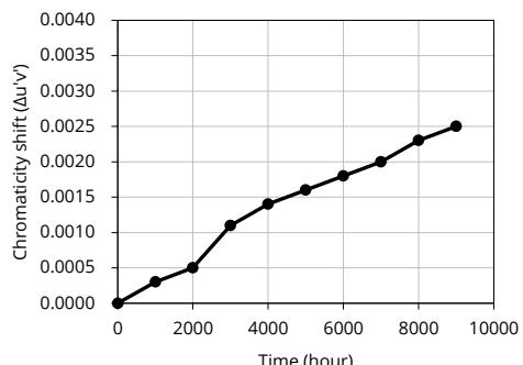
$T_s = 105^\circ\text{C}$ ,  $I_F = 300\text{mA}$ , RH < 65%, reported L70 > 54000 hours
