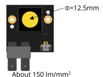
This is the ideal solution for applications requiring high power density. It can be widely used in professional stage lighting, photography lighting, cinematography lighting, or photoelectric device and relevant research.
