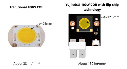
This is the ideal solution for applications requiring high power density. It can be widely used in professional stage lighting, photography lighting, cinematography lighting, or photoelectric device and relevant research.
