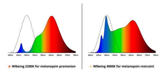
We develop and provide two essential spectrum theories of 2200K for melanopins promotion and 4000K for melanopsin restraint. The Wlbeing 2200K is designed as warm white for relaxing lighting environment. To promote the melanopsin secretion, the spectrum is designed to isolate the ipRGCs sensitivity limited to 26% proportion; the Wlbeing 4000K is designed as neutral white for focusing lighting environment. To restrain
