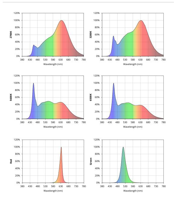
Typical spectral power distribution ( $T_A = 25$ °C,  $I_F = 150$ mA) (normalized) (continued)
