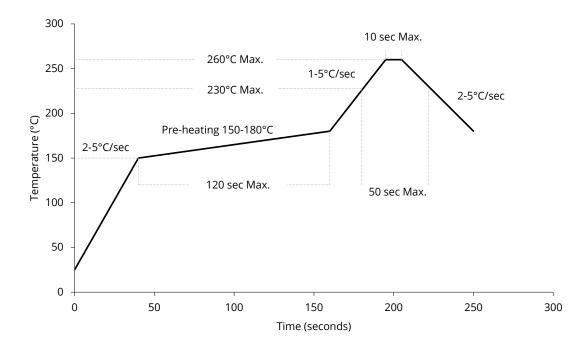
Note: Soldering paste with the melting point at 230°C is recommended.
