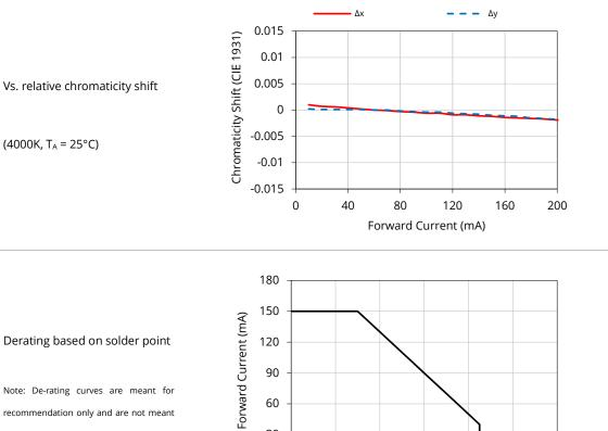
Note: De-rating curves are meant for recommendation only and are not meant to provide guarantees of product stability and longevity.
