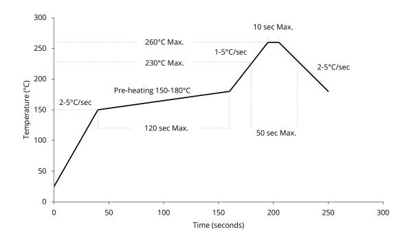
Note: Soldering paste with the melting point at 230°C is recommended.
