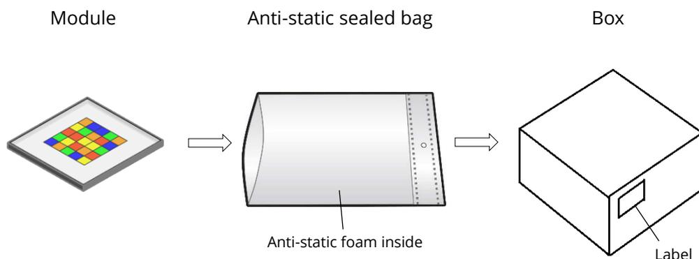
The size of box depends on the PCB size and production quantity.
